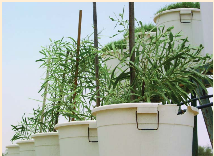
Lysimeter studies over time have given ICBA scientists significant data about salinity tolerance in a range of plants
